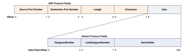
Your UDP protocol stack will take care of the first 8 bytes (0 to7) of the UDP protocol fields, which record the source and destination IP ports, the length of the datagram and a checksum over the entire datagram. The Data field (shown in blue), starting at offset 8 is where the Gemini protocol fields are located.
