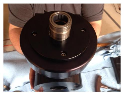
Photo 5. The bottom clutch plate is then installed.
