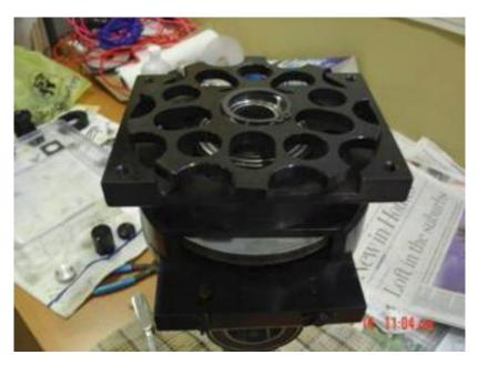
Photo 11. Snap ring shown before the pressure wheel is screwed down to permit installation. Photo from Titan Tips.
