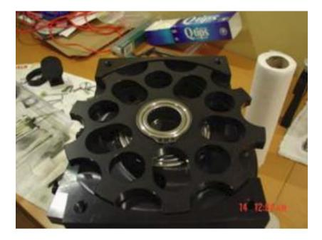
Photo 10. The pressure wheel is mounted. Screw it down far enough to permit the snap ring to be installed. Photo from Titan Tips.
