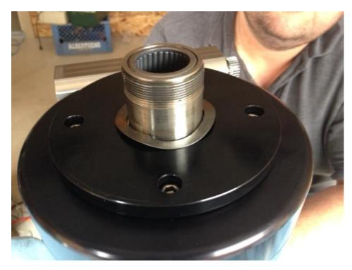
Photo 6. This is the first part of the installation that differs from Titan Tips. Compare to photos 8 and 9 below. The wavy washer is installed in the machined recess of the lower clutch plate BEFORE the installation of the clutch pad (see Photo 7).
