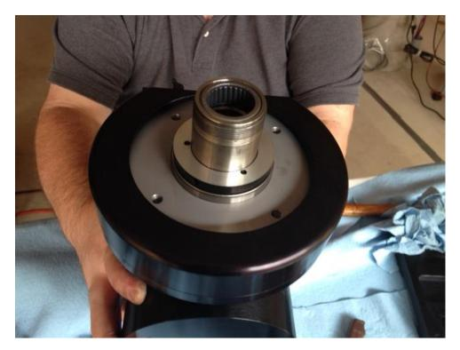
Photo 4. Gear housing fitted. Make sure that during installation you do not bump the gears.
