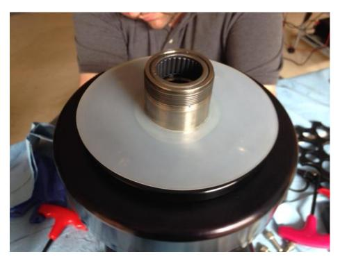
Photo 7. The clutch pad is installed directly over the wavy washer.
