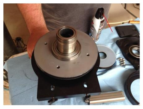
Photo 2. Dec gear placed on top of race bearing (again after clearing and lubricating).
