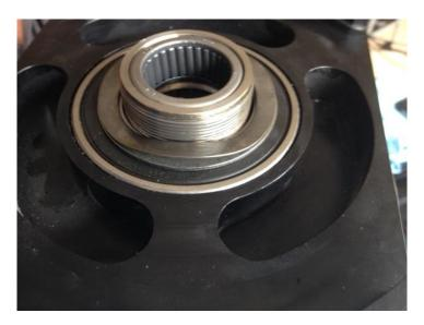
Photo 9. Detail of Photo 8. Again, ONLY the flat washer is installed, NOT the wavy washer and not two wavy washers. More explanation: If you try to install as in this photo, the pressure wheel does not work properly, it binds because there is not enough clearance once the snap ring is installed.
